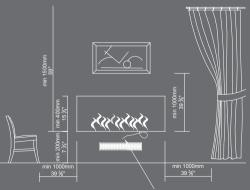
A power cable is required for connection to the mains. Specifica tion - min. 3x0, 75 mm2, with power supply 230 V, 50 Hz, to connect the device to the mains
