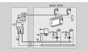
Boilers can be enhanced with mixer or hot water/mixer circuit controls (e.g. a Lago E8.0634 heating controller).
