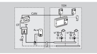
Combi boilers can be enhanced with mixer circuit controllers (e.g. E8.1124 mixer module).
