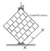
Figure 4 Diagonal tension strength
