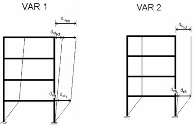
Figure 8 Structural ductility factors (left, VAR1); (right, VAR2)
