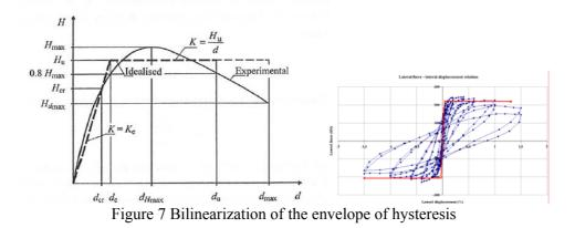
By taking a bilinear idealisation of the hysteresis envelope,  $H_u$  is evaluated by considering the equal energy dissipation capacity.
