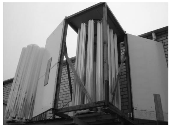
Figure 3. Evaporator of the heat pump covered with screens during the supply of warm air
